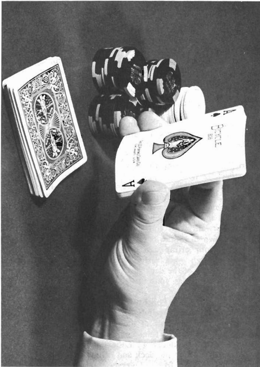
Figure 6 Flexing Cards Outward to Remove Crimp After Cutting
